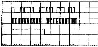
TOP IC101 pin 30 (DATA) MIDDLE IC101 pin 31 (CLK) BOTTOM IC101 pin 22 (LATCH) 5V/DIV. TB 50 \mu SEC/DIV.
